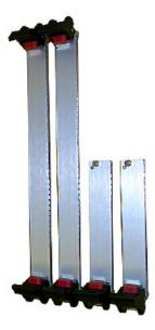
Panels are made from aluminium extrusion with a clear chromate finish and handles are plated die-cast zinc and UL94-VO plastic. All are compliant to IEEE1101.10/11
